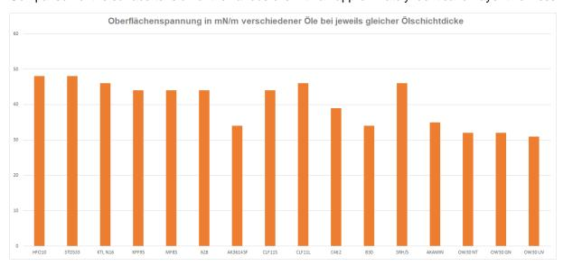
Investigation of the various oils has shown that the surface tension in similar oil layer thickness have different values depending on the respective oil.
