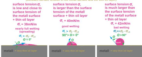
The test ink method is a simple and quick to implement procedure for the random testing of components. It would be preferable to obtain direct information about the residual oil layer thickness, which in the past has proven difficult to perform.
