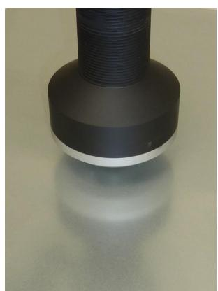
In order to ensure that environmental specifications are maintained during the application of the oils, and to ensure that the process is economical, it is advisable to ascertain the quantity of the oil applied. Oil quantity measurement can be performed inline, in a running process. UVA fluorescence measurement procedures are often used for this purpose. Not all oils exhibit the requisite fluorescence characteristics, and additional UV additives cause higher costs.
